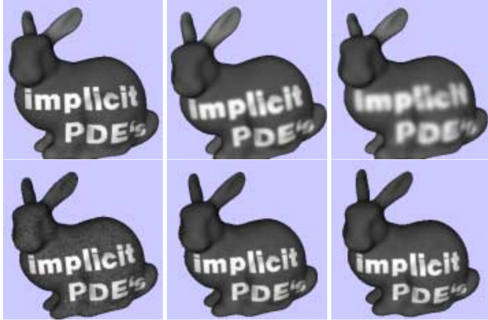
Figure 4.4: Intrinsic heat flow (first row, original, and 15 and 50 iterations respectively) and TV flow (second row, original, and 50 and 90 iterations respectively) for data defined on surfaces. Note how as expected, the heat flow blurs the data while the TV flow removes the noise while preserving the sharp edges (constraints on the noise have been added to the flow).
