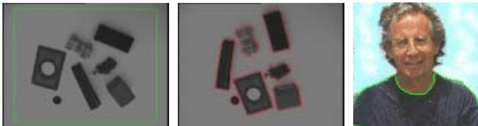
Figure 4.8: Level-set based object segmentation. The first figure on the left shows the original image and original contour, surrounding an un-known number of objects. The results of the geodesic active contours is given in the middle image. The properties of using the level-set framework are clear in this example. It not only allows for very accurate computations of geometric characteristics such as curvature but also freely permits topological changes, thereby detecting all of the un-known number of objects. The image in the right is a result of the geodesic active contours framework implemented following Cohen and Kimmel.
