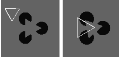
Figure 3. In these two graphs, the white curves represent the boundaries ( \varphi = 0 ) of the two different objective figures. The amount \int_R B(u)\varphi^2 dx dy for the right one is smaller than that of the left one, which means that the objective figure for the right case lies “closer” to the objects than the left one does, or closer to the desirable Kanizsa triangle in some sense.
