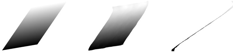
Fig. 5. Left: true depth map of the scene. Middle: recovered depth map. Right: profile of the recovered depth map. As can be noticed, the recovered depth map is very close to the true depth map with the exception of the top and bottom sides. This is due to the higher blurring that the images are subject to at these locations.
