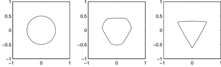
Figure 3: Evolution with surface energy defined by  $\gamma(\theta) = 1 + 3|\sin(1.5\theta)|$ , at  $t = 0, 0.016, 0.064$ .
