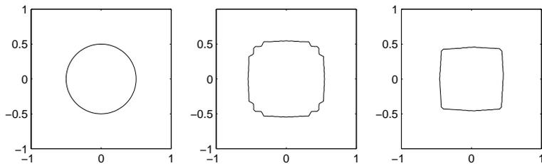
Figure 2: Evolution with surface energy defined by  $\gamma(\theta) = 1 + 3|\sin(2\theta)|$ , at  $t = 0, 0.016, 0.08$ .
