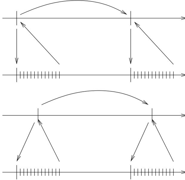
FIGURE 2.1. Schematic pictures of the interaction between the macro (upper lines) and micro (lower lines) scale computational domains for use with non-symmetric (top) and symmetric (bottom) kernels.
