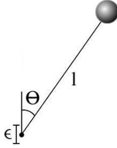
FIGURE 1.1. The inverted pendulum. A mass is connected to an arm of length  $l$  which makes an angle  $\theta$  with the vertical axes.
