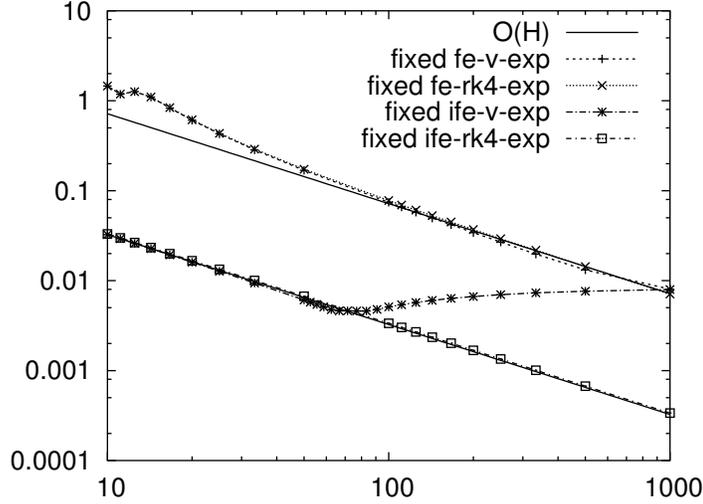
FIGURE 3.2. The error as a function of  $1/H$  for the first order schemes HMM-X-y, where X is FE or IFE and y is v or rk4. The width of the microscale domain and the step-size  $h$  are fixed with respect to  $H$ . The parameters used are listed in row two of Table 1. The slopes of the solid lines indicate decrease at first order in  $H$ .
