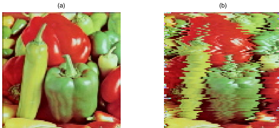
Figure 1: (a) an ideal image u(x, y) , and (b) its randomly jittered image u_J(x, y) .
