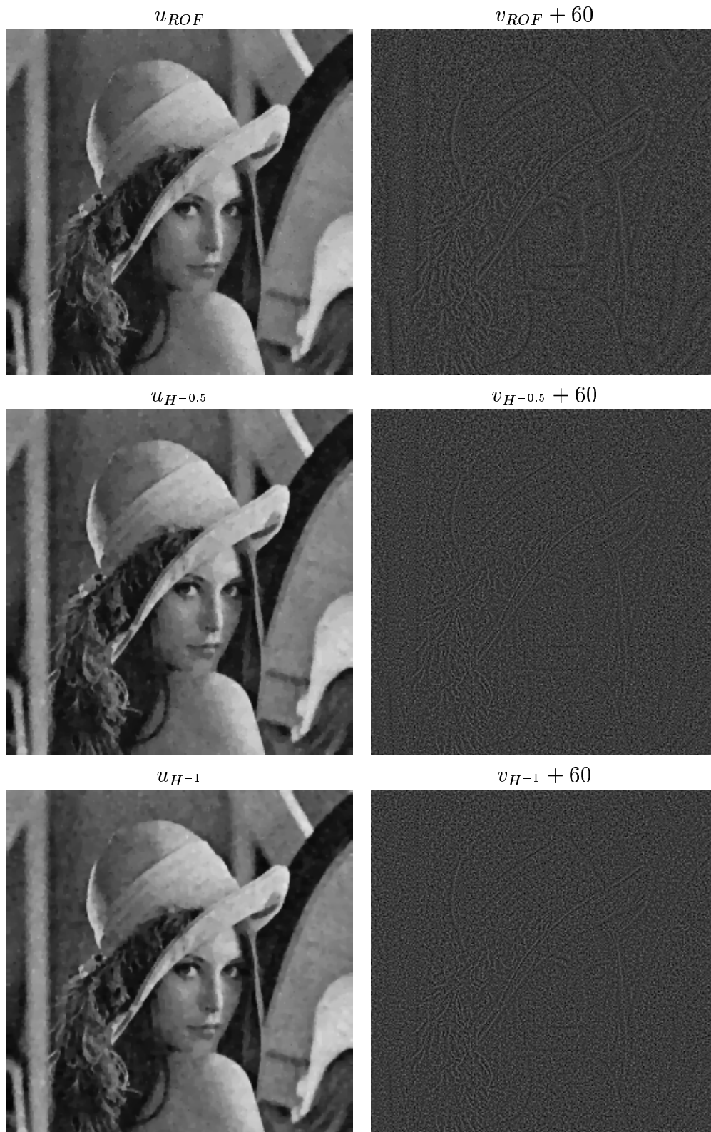
FIGURE 5. Denoising results on Lena image. Result of ROF model (top), result of our model with H^{-0.5} (middle), result of our model with H^{-1} (bottom).
