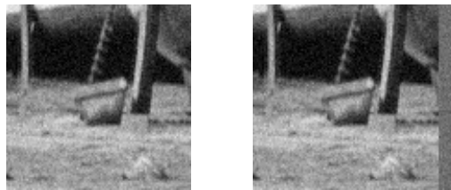
Fig. 1. Illustration of the direct (patch) method. Left: input image f . Right: a patch of pure noise with statistics similar to n is attached to the right side of f .
