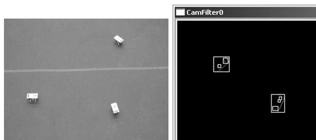
Fig. 2. (Left) An unprocessed shot of the testbed. (Right) Partial screen shot of the processed image. The large box surrounds the outer region of the vehicle. The medium size rectangle is the heading box. The small squares denotes the binary identification boxes. In the figure we see car #2 and car #3.
