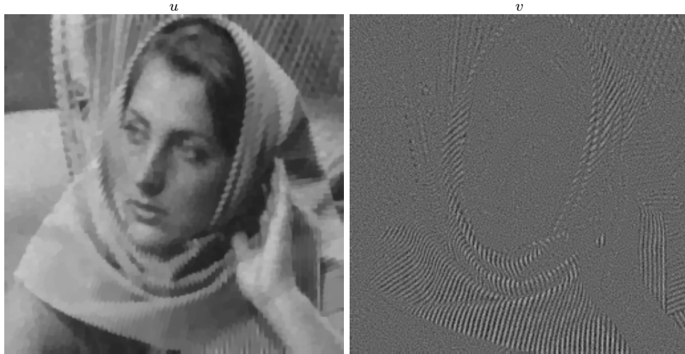
Figure 24: A decomposition of f_2 from Figure 2 using the model (59) with the kernel being the characteristic function of a disk centered at 0 having the radius equal to 1-pixel length, \varphi(\nabla u) = |\nabla u| , p = 1 , and \lambda = 1.5 .
