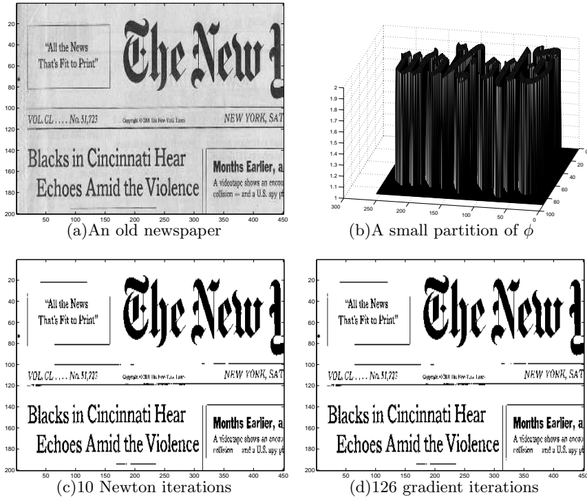
Fig. 2. A comparison Newton method with gradient descent method for the one-variable model. (a) An old real newspaper. (b) A small partition of the convergent \phi , it is a piecewise constant function \phi = 1 \vee 2 . (c) Segmented image using Newton method at 10 iterations, \beta = 0.1 . (d) Segmented image using gradient descent method at 126 iterations.
