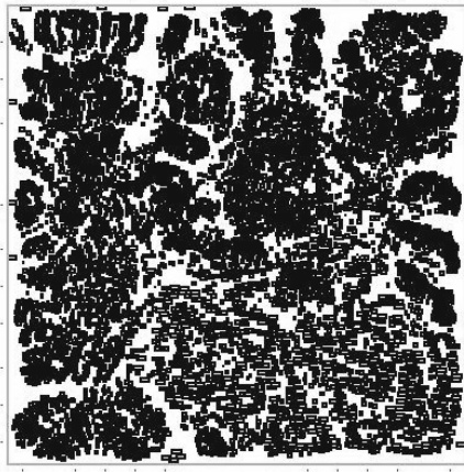
Figure 5.7: Global placement on a testcase ( \#cells = 12506 ) with utilization = 0.4. The half-perimeter wirelength is 2.2024 \times 10^6 .
