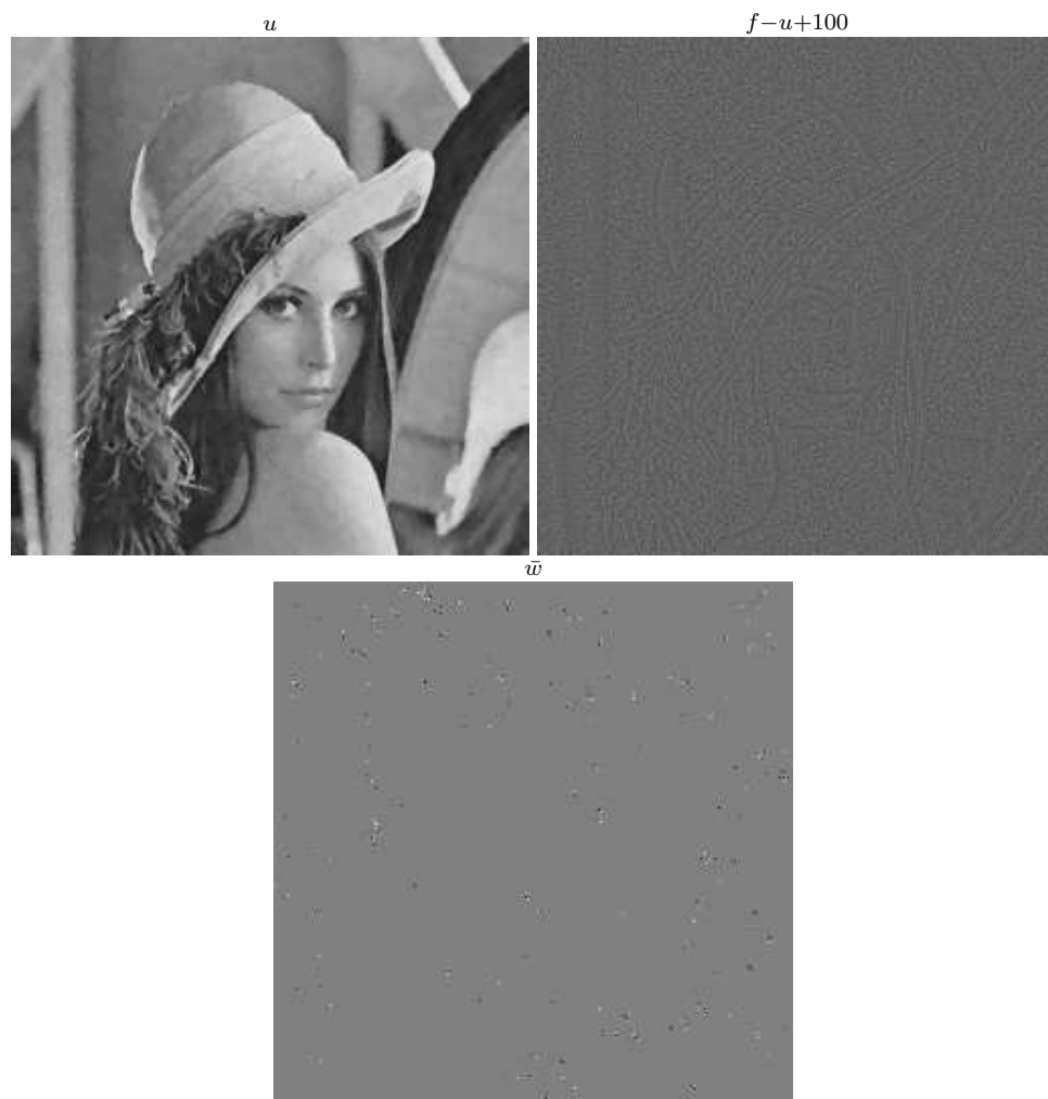
Figure 3.10: Denoising result of (\Phi, \Phi^*) model with non-convex \Phi in (3.20) applied to noisy image in Fig. 3.2(b), rmse = 0.02197276 , \lambda = 110 .
