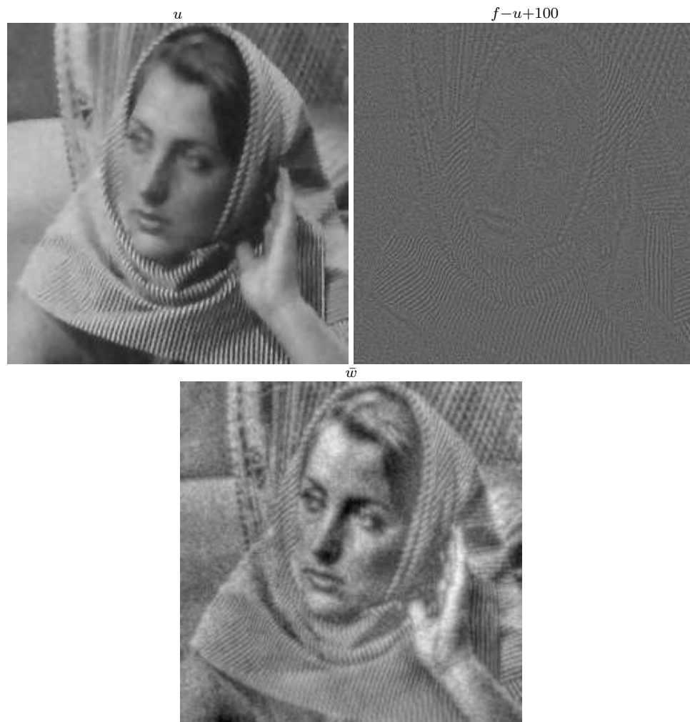
Figure 3.16: Denoising result of (\Phi, \Phi^*) model with non-convex \Phi in (3.21) applied to noisy image in Fig. 3.2(d) rmse = 0.04596249 , \lambda = 7 .
