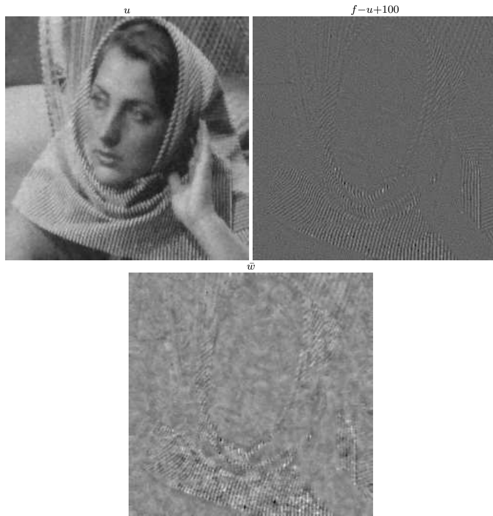
Figure 3.6: Denoising result of (BV, BV^*) model applied to noisy image in Fig. 3.2(d) using (3.14) and (3.15) with \lambda = 2500 .
