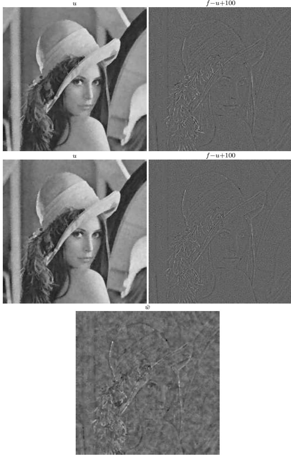
Figure 3.5: Denoising results of our proposed (BV, BV^*) model and ROF model applied to noisy image in Fig. 3.1(b). Top: ROF using (3.18) with \lambda = 63.75 . Bottom: (BV, BV^*) using (3.14) and (3.15) with \lambda = 2000 .
