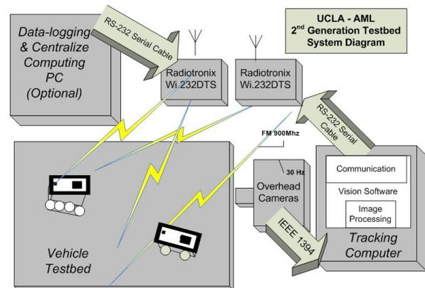
Fig. 1. Testbed System diagram
