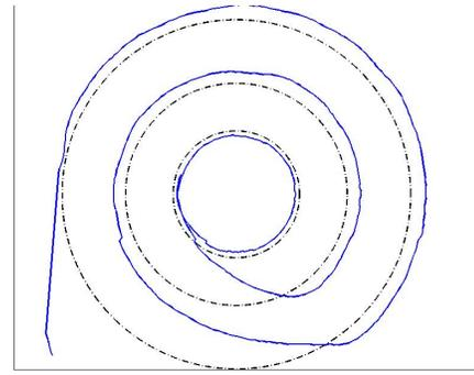
Fig. 7. A single car path (solid line) tracing, in sequence, concentric circles (dashed lines) of radii 65.5cm, 41.7cm, and 28.3cm.
