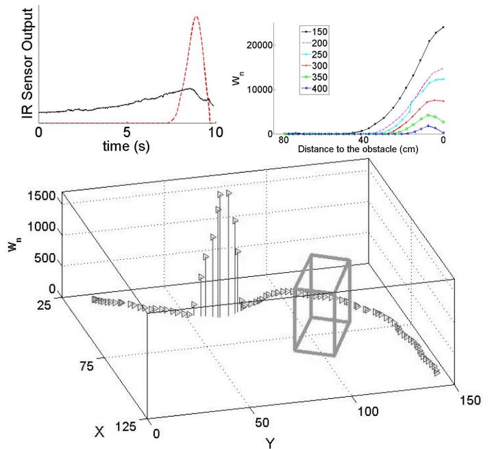
Fig. 10. Cumulative sum algorithm applied to sensor data from a single car approaching an obstacle. (top left) raw data and cumulative sum, (top right) cumulative sums for different choices of  $c$ , (bottom) sample car path avoiding obstacle with cumulative sum sensor output.
