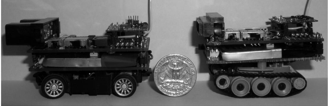
Figure 3.2: Left: car based vehicle; right: tank based vehicle.
