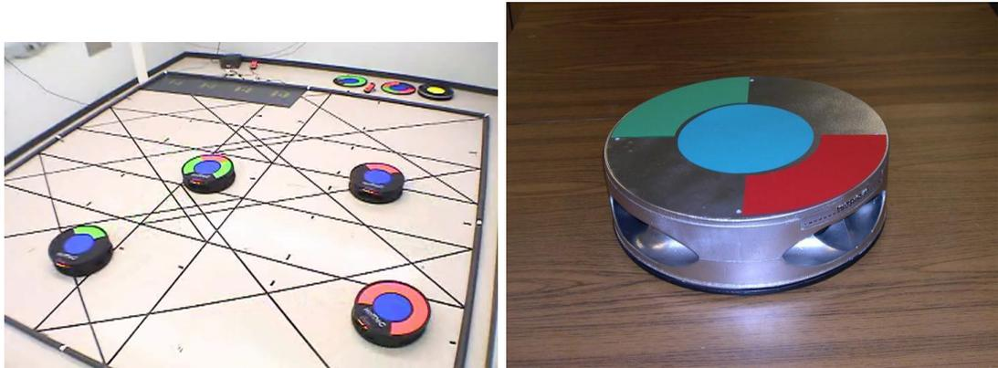
Figure 1.4: Left: a HoTDeC hovercraft; right: the HoTDeC testbed. Photo courtesy of University of Illinois at Urbana-Champaign Hovercraft Testbed for Decentralized Control.
