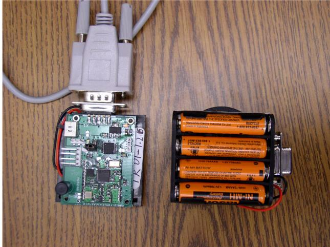
Figure 3.3: Front and back of the Wi.232DTS-integrated transceiver module connected to a RS232 cable
