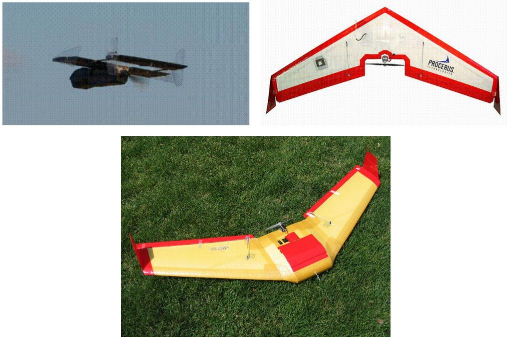
Figure 1.2: Top left: the MAV 06 Champion (wingspan 16 in); top right: the Unicorn (wingspan 48 in), a commercially available plane from Procerus technologies ([www.procerusuav.com](http://www.procerusuav.com)); bottom: the Bus (wingspan 60 in). Photo courtesy of the MAGICC Lab, Brigham Young University.
