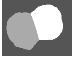
Fig. 3: The Euclidean influence zones f_{IZ} . The image in Figure 1(a) was used to create the marker image in Figure 1(c) where the three markers are uniquely labeled. Based on the distance transform, the Euclidean influence zones f_{IZ} were calculated to obtain an approximation on the boundaries of the finally segmented image. The influence zones are then later painted with at most four colors.
