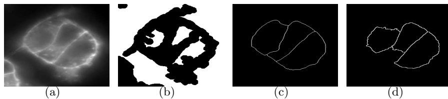
Fig. 5: Watershed segmentation of three cells and a background region. The image in (a) was used to automatically obtain markers (b) which were used for watershed segmentation by level sets (c) and for a standard watershed segmentation (d). Note that the watershed by level set captures more of the cells than the standard watershed segmentation.
