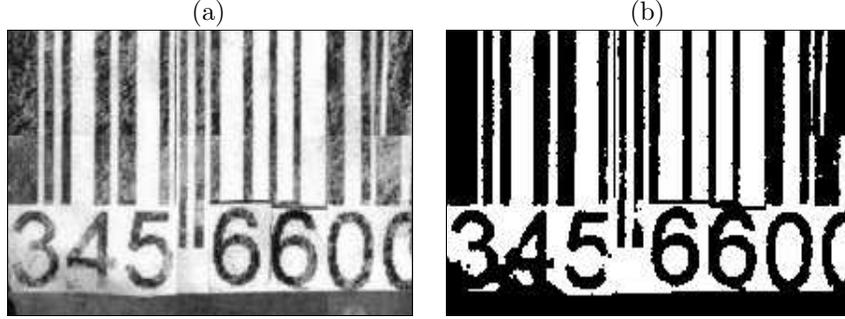
Figure 3: *Bar code processing: (a) noisy and moderately corrupted bar code image; (b) output from the quantum TV model.*
