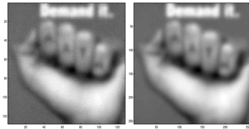
Figure 2: Left,  $128 \times 128$  low resolution degraded frame. Right, up-sampled and averaged image
