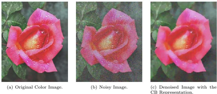
FIGURE 5. Application of the Chromaticity-Brightness (CB) color representation. Figure (c) presents the denoised color image with the CB representation. The SNR is 14.57 with the RGB color representation and 14.72 with the CB representation. (Note: All pictures are in color.)
