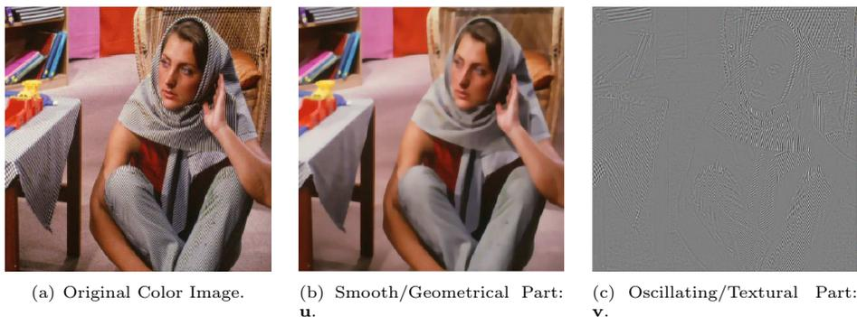
FIGURE 6. Color image decomposition process. Figure (b) presents the smooth/geometrical part of (a) and Figure (c) the oscillating/textural part of (a). The decomposition process takes 19sec and 60 iterations. The picture size is 512x512. (Note: All pictures are in color.)
