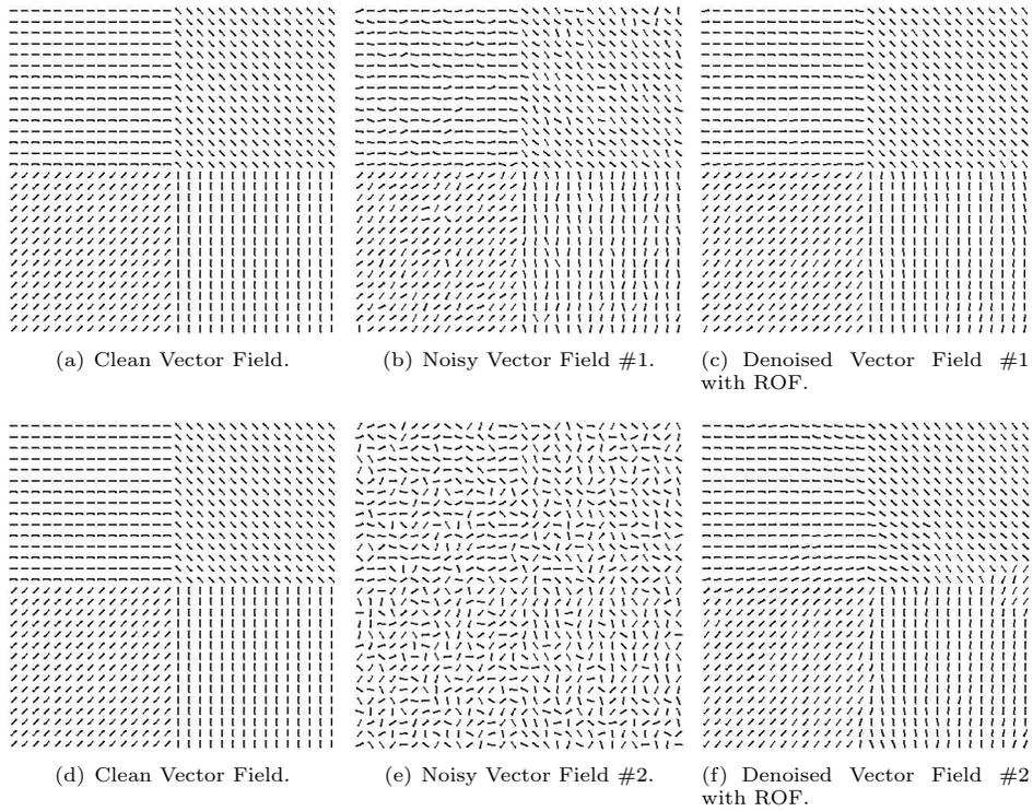
FIGURE 11. Denoising of a vector field with the vectorial ROF model. The denoising process takes less than 0.1sec, 30 iterations for #1 and 100 iterations for #2. The picture size is 30x30. We can notice the good performance of our denoising model with the noisy vector field (e), which has lost the main directions (d). Our model is able to recover the main structure (f).
