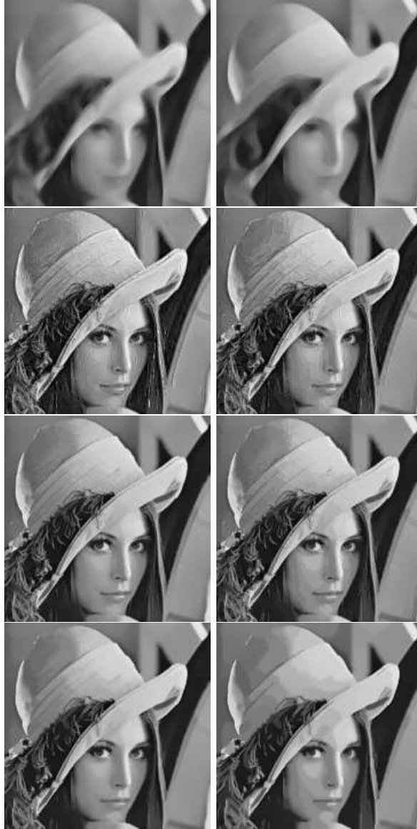
Figure 7: Comparison of linear (left images) and nonlinear (right images) diffusion schemes. From top to bottom: original image, mean curvature motion, the Perona-Malik equation, the sigma filter and the NL-means. This experiment shows first that linearized versions are more faithful for the original. This is not a surprise, since the original image features are kept in the linearized version while they are updated in the nonlinear version. The third row illustrates how much better the linearized version of the neighborhood (or sigma-, or bilateral) filter performs with respect to the non linear one. We observe the same effect in the NL-means algorithm. The iterated version produces shocks as the neighborhood filter, which are avoided by its linear counterpart. See Section 3 for more details.
