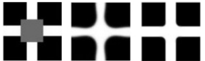
Fig. 4. Cahn-Hilliard vs. wavelet inpainting (left to right): the input image, CH inpainting (for two stages respectively: \epsilon^{-1} = 1 and 100 , \mu = 3 \times 10^5 and 10^7 , 500 iterations for each stage), wavelet-based inpainting \epsilon = 1/32 , \mu = 100 , 72 iterations.
