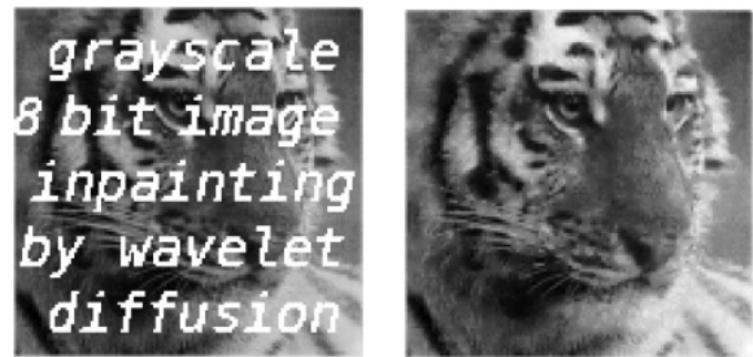
Fig. 7. Grayscale inpainting under occluding text. 8-bit image(16 gray levels) is inpainted after 40 iterations (using Daubechie’s 7/9 wavelet).
