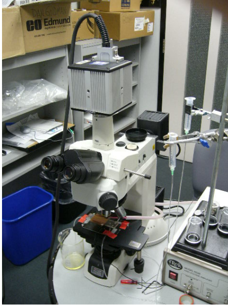
Figure 5.3 The microscope/high-speed camera set-up.
