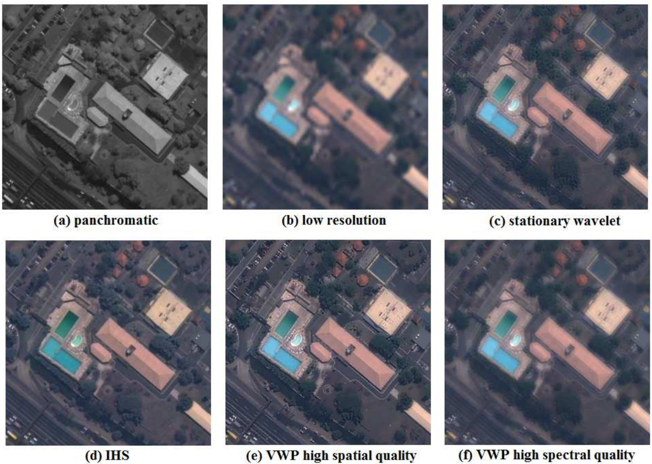
Fig. 4. Results of different pan-sharpening methods; (a), (b): Copyright DigitalGlobe, NextView liscense, 2003; image (e): parameter choice (2), image (f): parameter choice (1)
