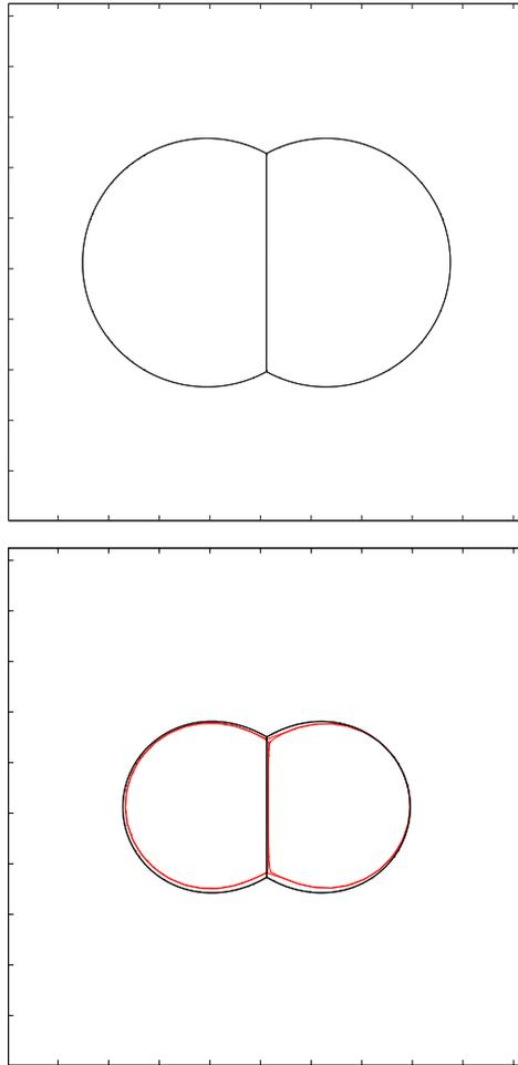
Figure 12: The first plot shows the initial condition for algorithm (92) & (93). The second plot shows the solution at  $t = \frac{1}{64}$  computed using 30 time steps at  $32 \times 32$  spatial resolution (red curve), superimposed with the computed result using 480 time steps at  $512 \times 512$  resolution (black curve). The error in the latter is about one thirteenth of the former.
