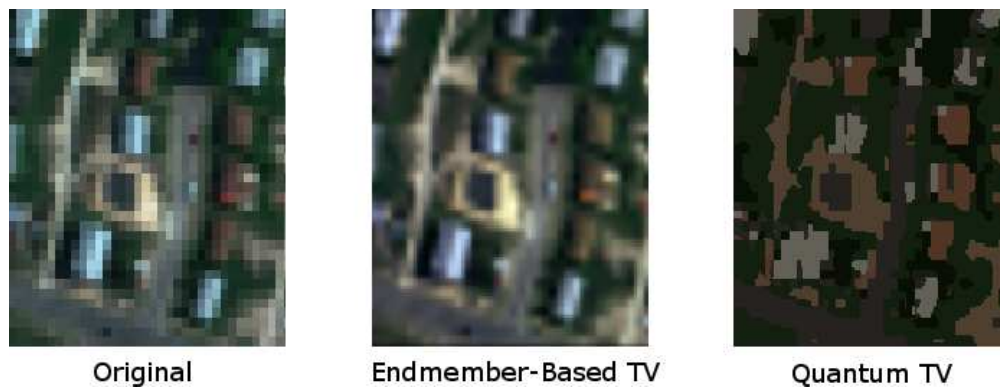
Figure 5. Enhancement of portion of the 163-band Urban image with 4x zoom - displayed as false color RGB image.
