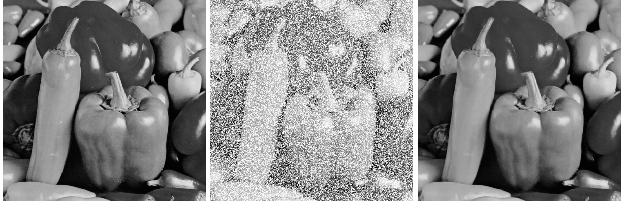
(a) The 512 \times 512 “peppers” image. (b) 50% pixels are randomly missing. (c) Recovered by (1.7). The algorithm employed is the split Bregman method in [13].
