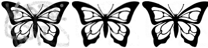
FIGURE 5. Destroyed binary image and the solution of Cahn-Hilliard inpainting with \lambda_0 = 10^9 and switching \epsilon value: u(800) with \epsilon = 0.8 , u(1600) with \epsilon = 0.01
