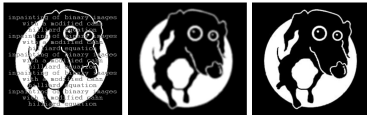
FIGURE 4. Destroyed binary image and the solution of Cahn-Hilliard inpainting with \lambda_0 = 10^9 and switching \epsilon value: u(200) with \epsilon = 0.8 , u(500) with \epsilon = 0.01
