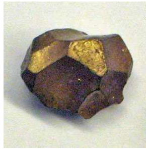
Figure 2: A single grain of beta brass, approximately 2 cm in diameter, from the collection of W.W. Mullins. The photograph is due to K. Barmak and D. Kinderlehrer. The grain compares well to the simulated grain shown in Figure 1.
