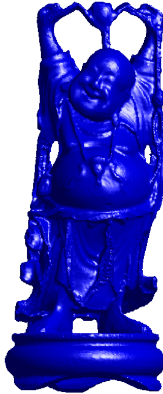
Fig. 7. Three dimensional multigrid narrow band surface reconstruction for Buddha on 149 \times 365 \times 149 grid. The point cloud contains 144647 points.
