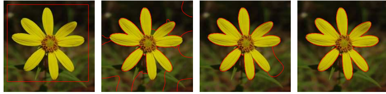
Fig. 5. The result of our method for a color image of flower. It shows the curve evolution process from the initial contour to the final contour
