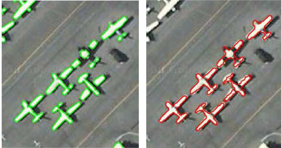
Fig. 4. Segmentation of multiple objects in hyperspectral image of Santa Monica Airport. Left: Segmentation without priors. Right: Segmentation using a metal signal prior and the airplane shape prior.
