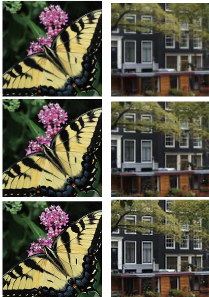
Fig. 2. From top: Upsampled images ( \times 2 ) resulting from bilinear, b-spline, and edge-preserved interpolation applied to the downsampled original image. The same interpolation method is applied separately to each of the luminance and the two chrominance channels.
