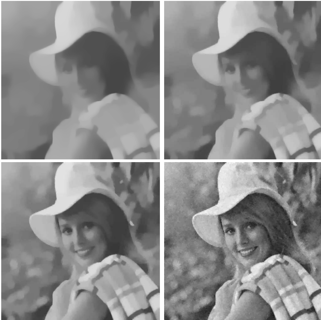
Figure 8: (Example 5.4) (From left to right, top to bottom) Steady state solutions using the proposed ADE scheme with \Delta t = 40\Delta x^2 and \lambda = 0.005, 0.010, 0.020 and 0.050 .
