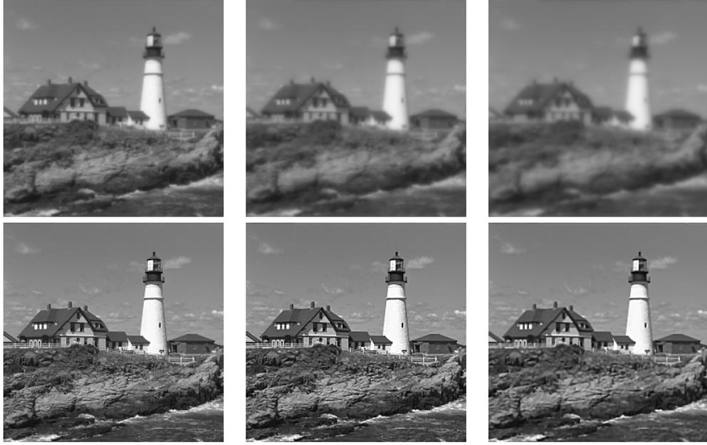
Figure 11. Blurred and blind Fried deconvolved images (first column:  $C_n^2 = 1.5 \times 10^{-14} m^{-2/3}$ , second column:  $C_n^2 = 7.6 \times 10^{-13} m^{-2/3}$ , third column:  $C_n^2 = 13.8 \times 10^{-13} m^{-2/3}$ ).
