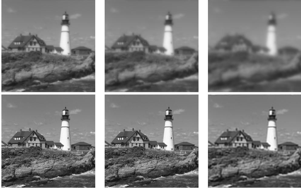
Figure 3. Blurred and nonblind Fried deconvolved images (first column:  $C_n^2 = 7 \times 10^{-14} m^{-2/3}$ , second column:  $C_n^2 = 2 \times 10^{-13} m^{-2/3}$ , third column:  $C_n^2 = 5 \times 10^{-13} m^{-2/3}$ ).
