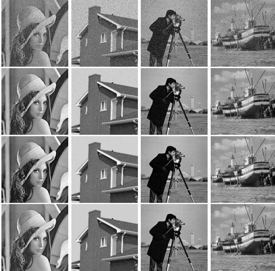
Fig. 5.2: Denoising results of images contaminated by both Gaussian noise and random-valued impulse noise with \sigma = 10 and s = 25\% . Top row: noisy images; Second row: the results restored by ACWMF; Third row: the results restored by TVL1; Bottom row: the results restored by total variation blind inpainting using AOP.
