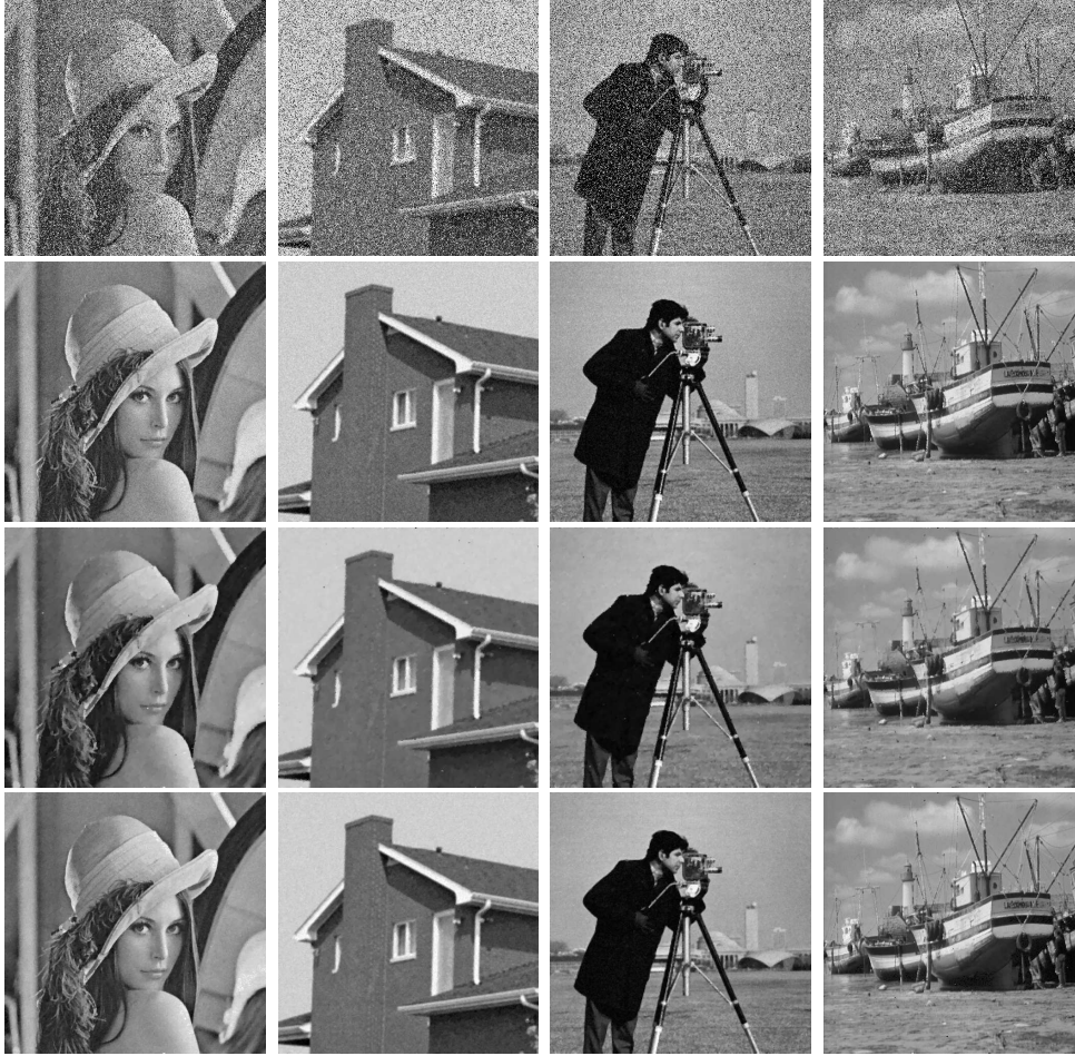
Fig. 5.1: Denoising results of images contaminated by both Gaussian noise and salt-and-pepper impulse noise with \sigma = 10 and s = 30\% . Top row: noisy images; Second row: the results restored by AMF; Third row: the results restored by TVL1; Bottom row: the results restored by total variation blind inpainting using AOP.
