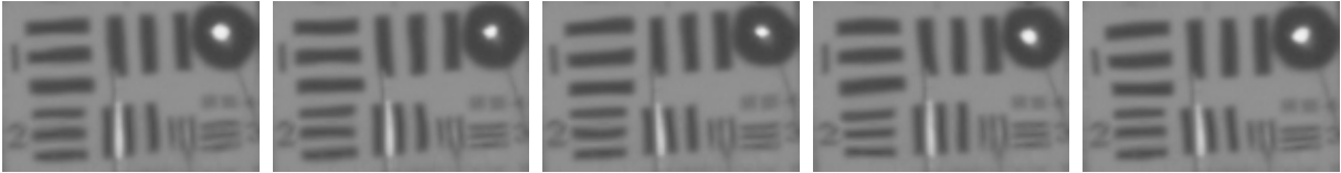
Figure 6: Frames obtained by warping the centroid via a synthesized sequence of optical flows ( n = 50 , \tau = 200 ); the images in each consecutive pair above are 8 time samples apart.
