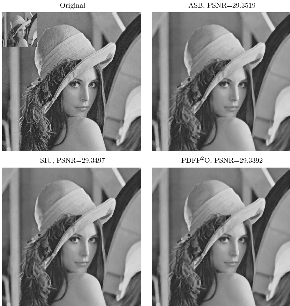
Figure 5.2: Super resolution results from 128 \times 128 image to 512 \times 512 image by ASB, SIU and PDFP 2 O; noise level \sigma = 1 .
