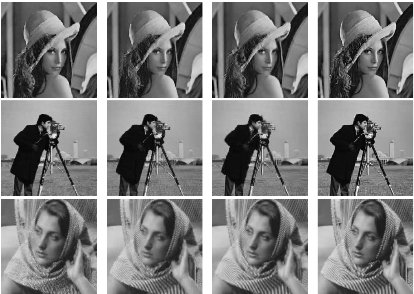
Fig. 6. The inpainted images for the images of “Lena”, “Cameraman”, and “Barbara” (from top to bottom) corrupted by impulsive noise with noise level of 70%. The results (from left to right) are produced by SF, SF-LDCT, MCA, and Algorithm 3, respectively.
