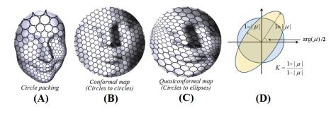
FIG. 2.1. (A) shows a human face with circle packing texture. Under the conformal parameterization, infinitesimal circles are mapped to circles as shown in (B). Under quasi-conformal parameterization, infinitesimal circles are mapped to ellipse as shown in (C). (D) illustrates how the Beltrami coefficient measure the conformality distortion of a quasi-conformal map.
