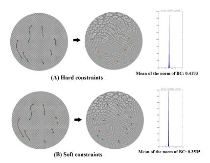
FIG. 6.7. T-Map with soft landmark constraints. (A) shows the obtained T-Map with hard landmark constraints. The histogram of the norm of BC is plotted, which is accumulated at 0.4193. (B) shows the obtained T-Map with soft landmark constraints. Landmarks cannot be exactly matched, but less conformality is introduced, as shown in the histogram of the norm of the BC.
