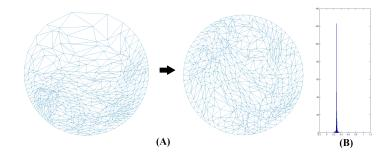
FIG. 5.4. Computation of T-Map on an irregular mesh. The QC iteration is independent of the mesh structure. The boundary condition is given and the associated T-Map is constructed, as shown in (A). (B) shows the right shows the histogram of the norm of the BC.
