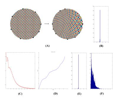
FIG. 5.5. T-Map of the disk with only 8 landmark points constraints on the boundary. (A) shows the T-Map. (B) shows the histogram of the BC norm. (C) shows the sup-norm of the BC in each QC iteration. (D) shows the automatically obtained optimal boundary correspondence. (E) shows the histogram of the BC norm under the T-Map with arc-length parameterized boundary condition. (F) shows the histogram of the BC norm under harmonic map with arc-length parameterized boundary condition.
