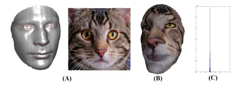
FIG. 7.3. (A) shows a human face and a texture image of a cat. Corresponding landmark points are labeled on the surface and the texture image. We compute the T-Map that matches the landmark points. The T-Map is used as constrained texture mapping to project the texture image onto the surface, as shown in (B). (C) shows the histogram of the norm of BC.
