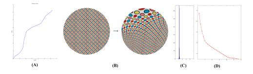
FIG. 5.2. Example of the T-Map of the disk with fixed Dirichlet boundary condition. (A) shows the boundary condition. (B) shows the obtained T-Map, visualized using the texture mapping. (C) shows the histogram of the BC norm. (D) shows the sup-norm of the BC in each QC iterations.
