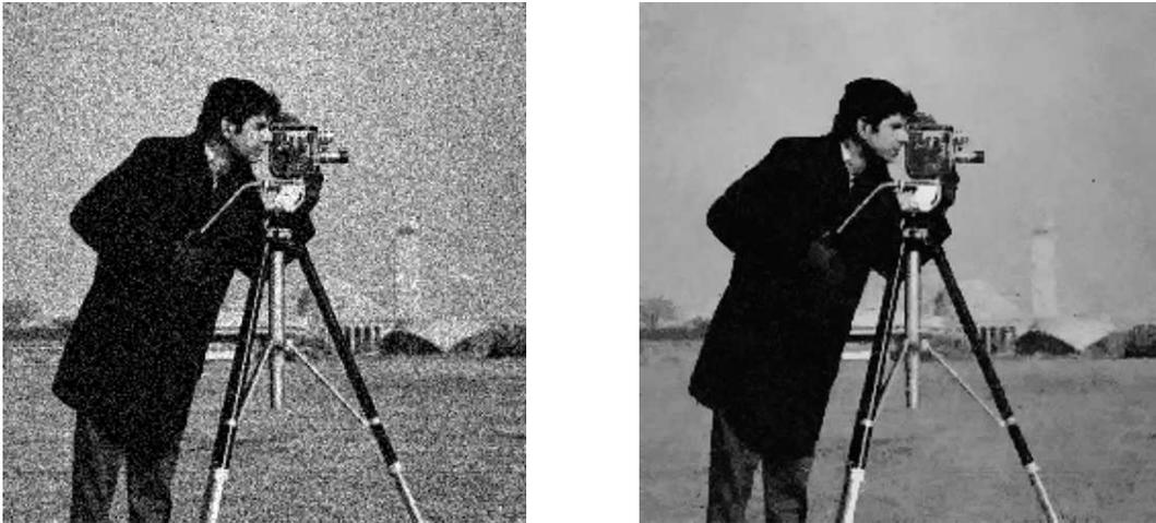
Figure 5: Left: input noisy image with mixed Poisson-Gaussian noise, peak intensity: 120, PSNR: 18.59dB; right: denoised by model (31), PSNR: 27.42dB.
