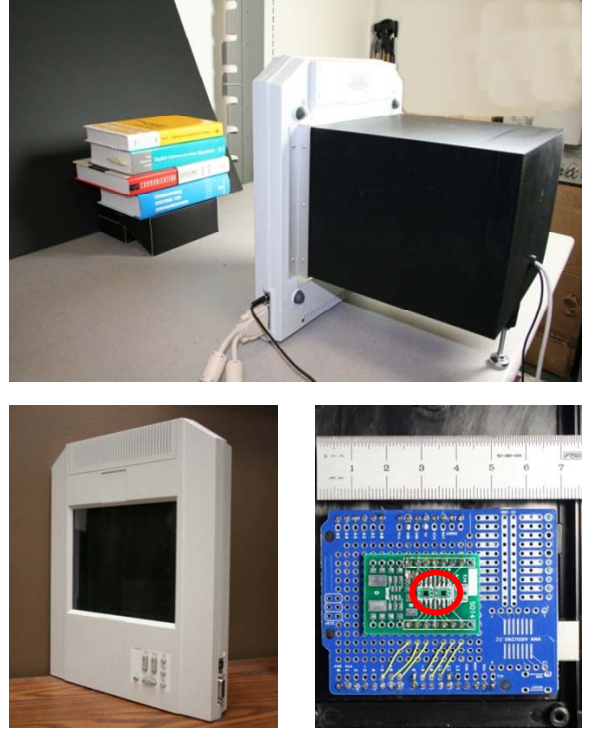
Figure 9. Prototype device. The top photo shows the laboratory set up to acquire the image of the books. The bottom left is the LCD screen used as the aperture assembly, and the bottom right is a photo of the RGB sensor board. Two sensors, indicated by the red circle, are mounted on the board.
