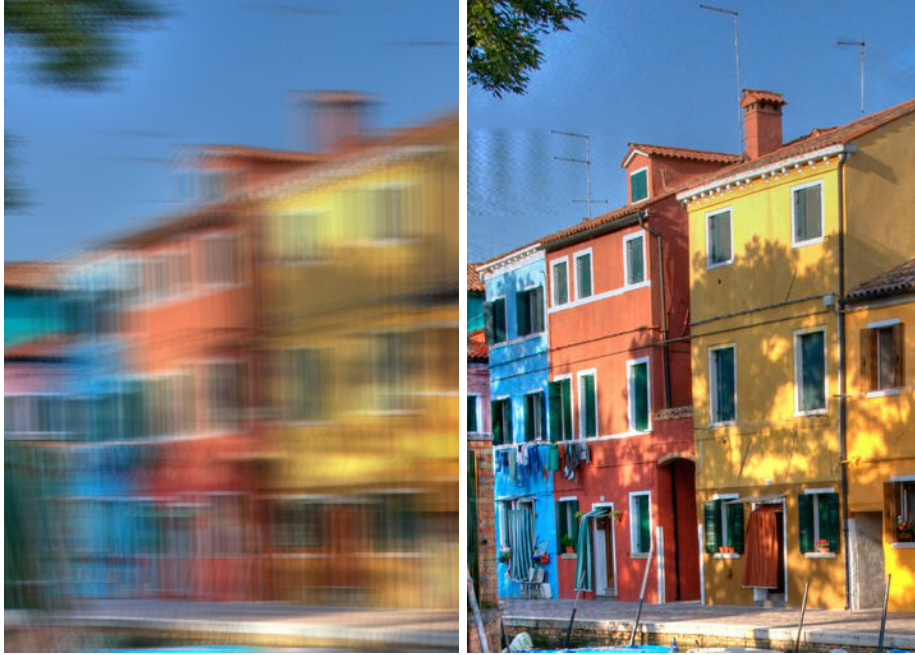
Figure 1: Simulated observed (blurry and noisy) image (left). The blur interval length is 52 pixels. Notice the stroboscopic effect of the flutter shutter apparatus. Reconstructed image (right). Such reconstruction is not possible without a flutter shutter camera.
