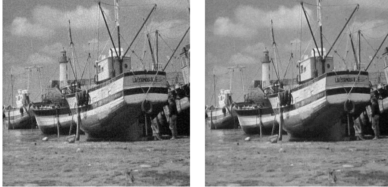
FIG. 2.1. Image denoising comparison of two methods: (left image) solving (2.3) with all patches used at once, (right image) solving (2.3) with one subset of non-overlapping, covering patches. In (2.3), \nu = 0.05 , and \mathbf{D} was learned according to section 4.2.
