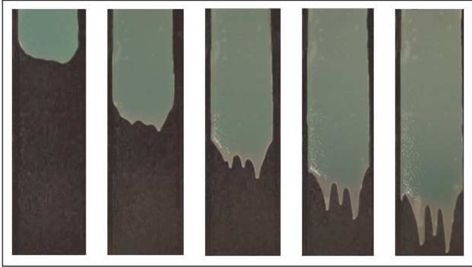
Fig. 9 Pictorial evolution of the ‘settled’ regime showing the particles settling while clear fluid flows over the particles resulting in the formation of fingers. The plane angle of inclination is set to 30^\circ while the particle concentration is chosen as 0.25. The first snapshot is shown 30 seconds after the onset of the experiment while the last one is shown after 3 minutes. The color of the inclined plane has been darkened to clearly show the contrast between the particle-rich region (light blue) and the clear fluid fingers.
