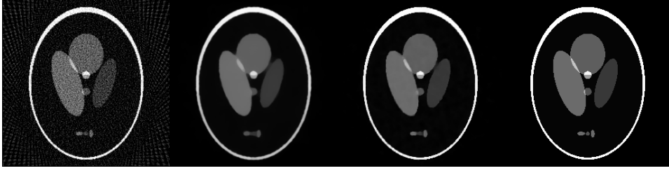
FIG. 5.1. The SNR = 24.7dB. From left to right, reconstructed images by FBP, the proposed method, SFEM, and the original image with gray scale over [0.0, 1.0] .
