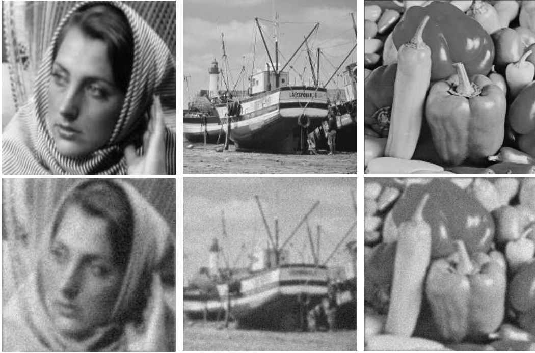
Figure 1: Test images: original (first row) and observed (second row). The PSNR values of the observed images are 23.4519 (Barbara), 22.4428 (Boat) and 22.5482 (Peppers). The image size of “Barbara” is 195 \times 195 , and both “Boat” and “Peppers” has size 256 \times 256 .
