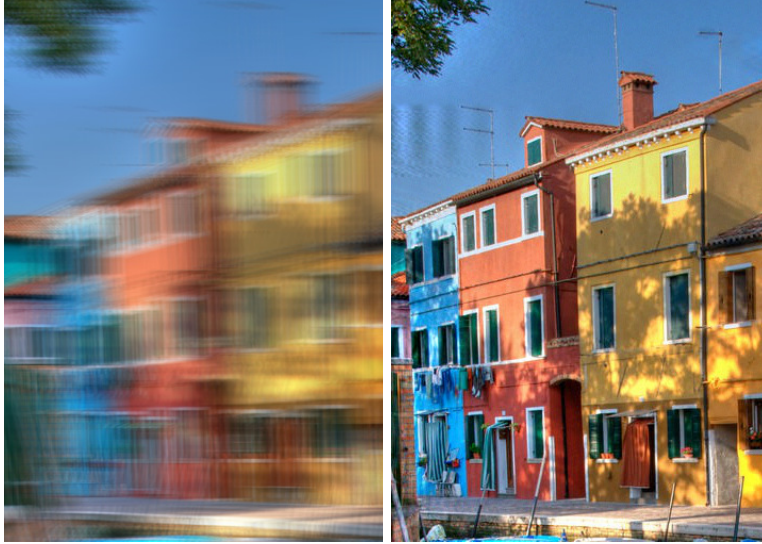
Figure 1: On the left panel: simulated observed (blurry and noisy) image using the Agrawal, Raskar et al. [1]. The blur interval length is 52 pixels. Notice the stroboscopic effect of the flutter shutter apparatus. On the right panel: the reconstructed image obtained by a direct deconvolution. See [33] for a peer reviewed implementation and on line demonstration of a flutter shutter camera simulator.
