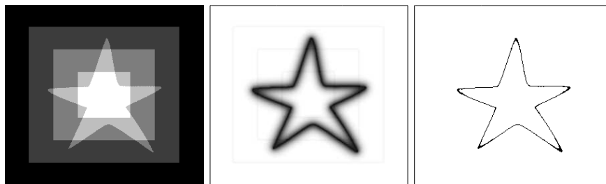
Fig. 3 From left to right: the input image which has a star occluded partially by the background, the output edge strength function v , and the extracted boundary.
