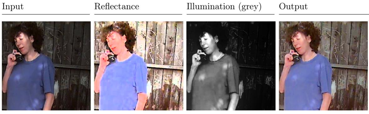
Figure 7.3: **HSV color Retinex.** Retinex is performed on the value-channel of a color image in HSV space. The final output is obtained by applying post-processing enhancement as in [36].
