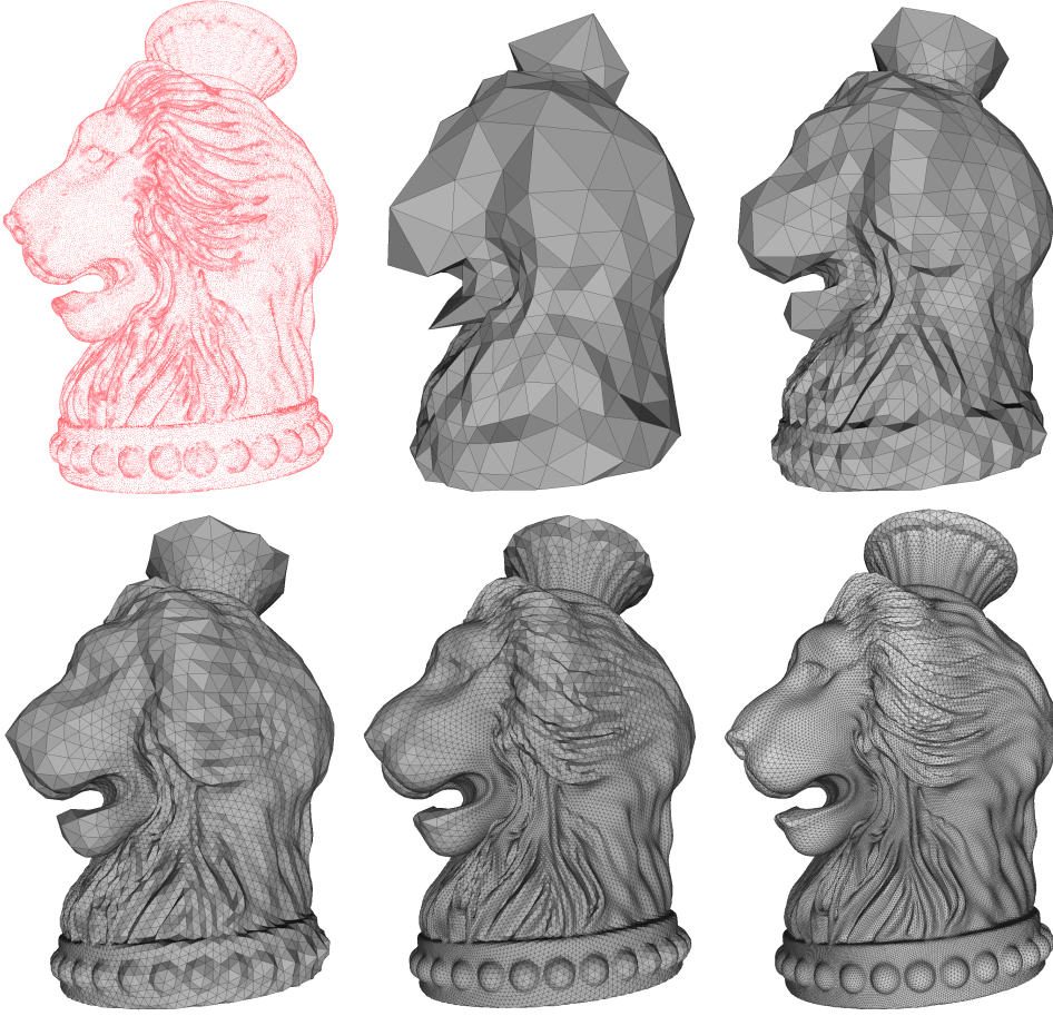
FIG. 7.12. Multilevel representations of a genus-0 lion vase point cloud. For better visualizations, we create mesh structures on the representations. Top left: a lion vase point cloud with 256094 points. Top middle to Bottom right: the multilevel representations with 0, 1, 2, 3 and 4 subdivisions. The representations are with 696, 2778, 11106, 44418 and 177666 points respectively.
